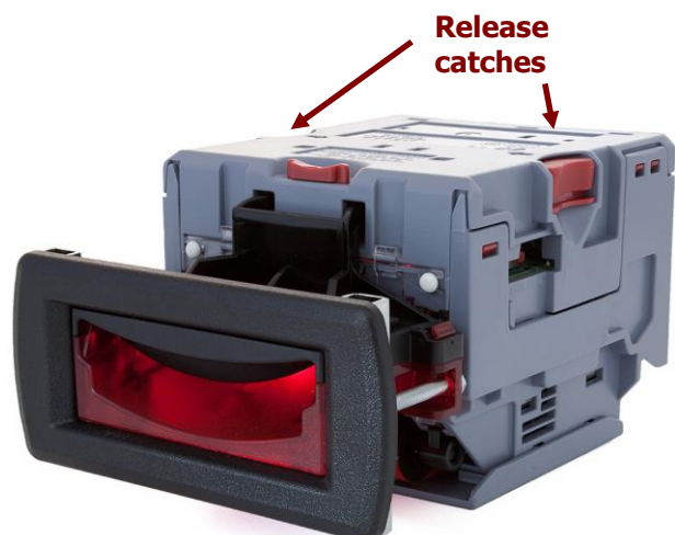
Figure 10 – NV10 USB Release Catches
