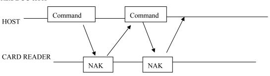
Card reader received a communication package and BCC is error, send NAK to HOST to show BCC error. Host need check its communication package BCC is correct or not. Resend it after checking is correct. Card reader will not send ACK to HOST until it receives that communication package BCC is correct.
