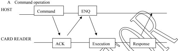
Host sends command, Reader receives and checks if BCC is correct. Host sends ENO after return ACK, Reader will execute the relevant operation and return relevant operation information to host according the command.
