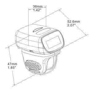
Figure 1-1 Dimensions of the scanner
