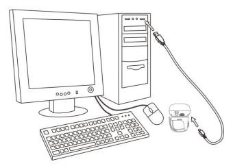
Figure 2-1 Diagram of connecting the scanner to PC
